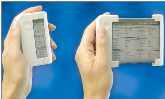
The Philips READIUS has a rollable display that lets you carry around a much larger screen in a pocketable form factor
