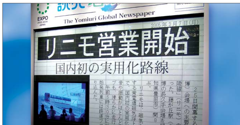
This is a wall-sized paper display that was set up at an exhibition in Japan. It used E-Ink's technology to display newspaper articles on the paper display, while images were displayed on the smaller LCD
